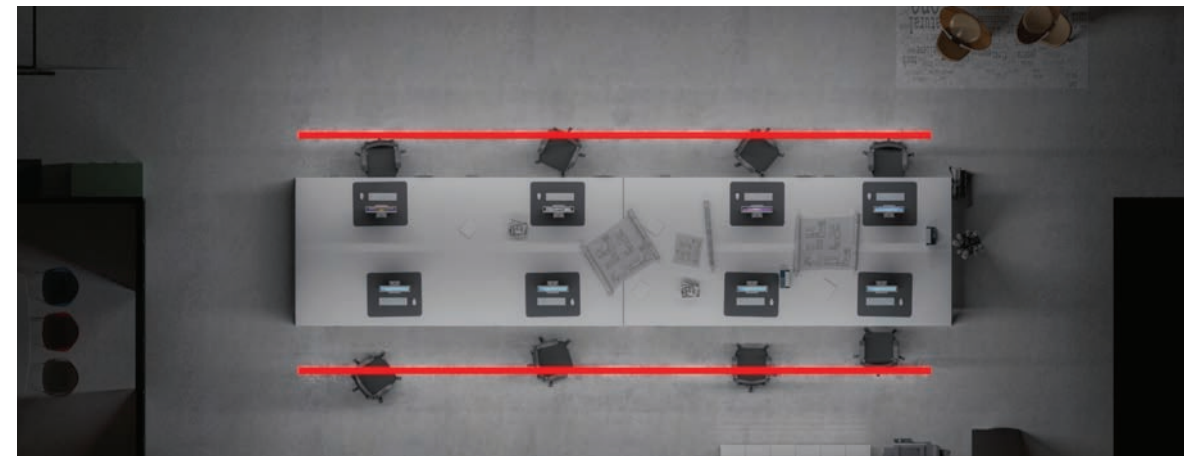
Emergency layout with Modulus allows for a more balanced approach to emergency lighting, with the ability to specify all or multiple lit sections for a more uniform distribution.
